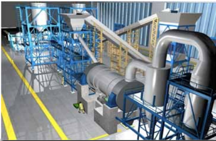
CERL's net-zero support includes a project to evaluate waste-to-energy options, such as this conceptual graphic of a rotary kiln waste gasification system under construction at the State University of New York. Graphic courtesy of W2E Ventures, Inc.
