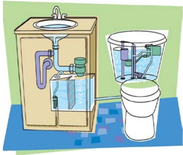
Technologies to capture, filter, and reuse graywater are commercially available, such as this unit that catches water from lavatory use and recycles it for toilet flushing. Photo courtesy of WaterSaver Technologies. Used with permission.
